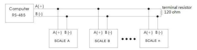
NOTE: when connect with multiple devices, parallel a 1200hm resistor in the last device
